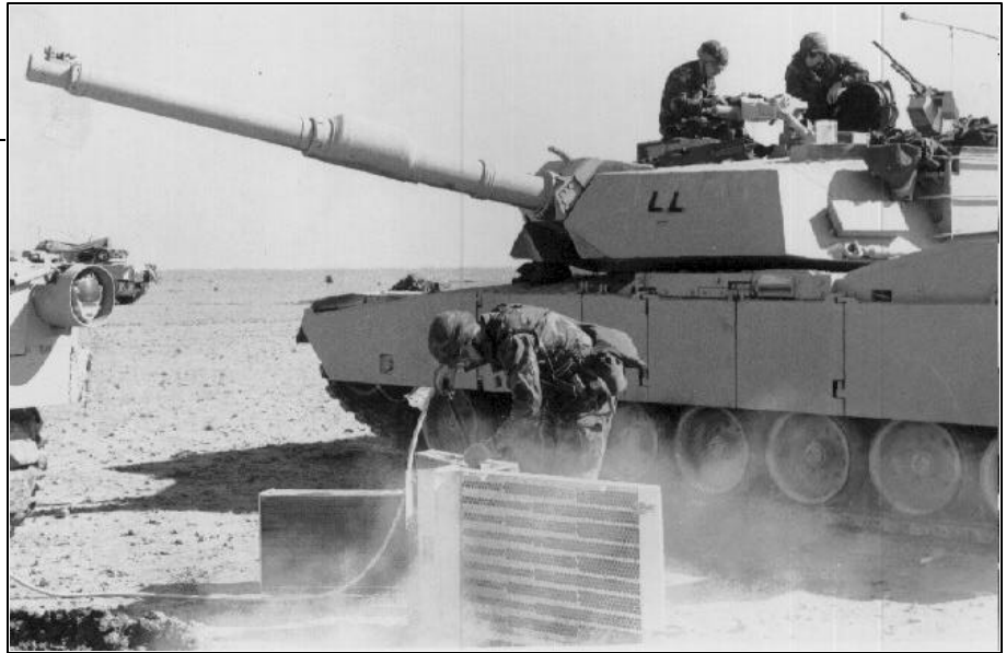
3rd Armored Division tankers pause to blow out their air cleaners during Desert Shield.
