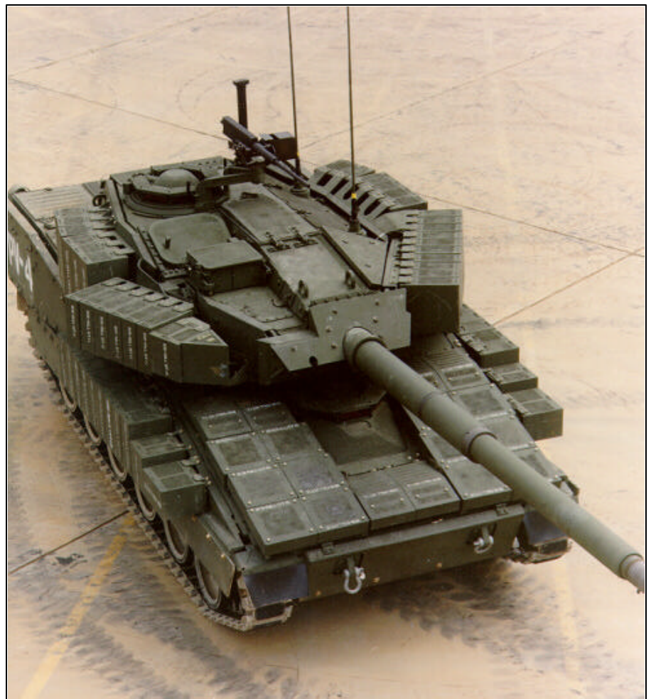
The AGS light tank system, shown here with the heaviest of its three levels of add-on armor, was intended as a replacement for the M551. It was designed to be delivered by air to provide 105mm firepower for light forces. But after several prototypes were built and testing had begun, the project was canceled to save money.
